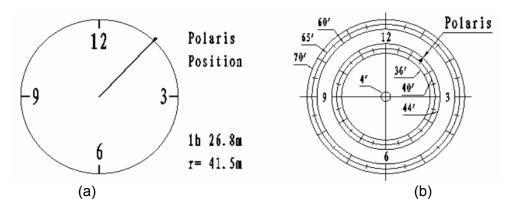
Figure 24. Polaris Position shown on HC (a) and where to put on polar scope dial (b)
